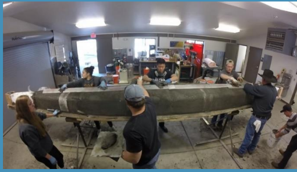
Figure 17: Apply Reinforcement over Ribs & Center
