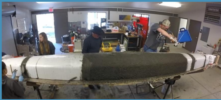
Figure 16: Spray 1/8" Concrete onto Mold
